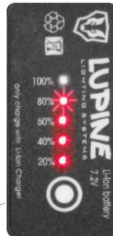
**Example:** 3 LEDs steady glow (20 %, 40 %, 60 %) = 70 % remaining capacity
